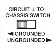
The ground-lift switch allows eliminating noise loops. If the power amplifier is operated together with other equipment in a 19" rack-shelf, setting the switch to its GROUNDED position is recommended. If the power amplifier is operated together with appliances with differing ground potentials, setting the switch to its UNGROUNDED position is recommended.
